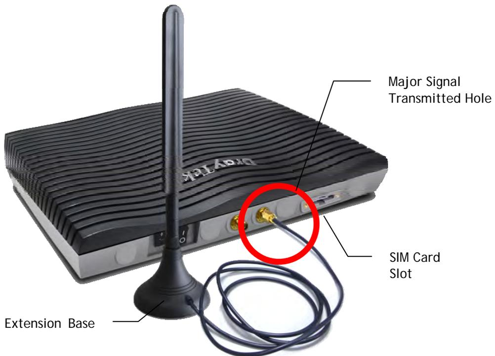
Note, if only one antenna shall be installed, please use the mounting hole (major signal transmitted hole) near to the SIM card slot.
