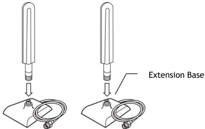
There are two mounting holes for installing antennas with extension base on Vigor router. Please install them as shown below.
